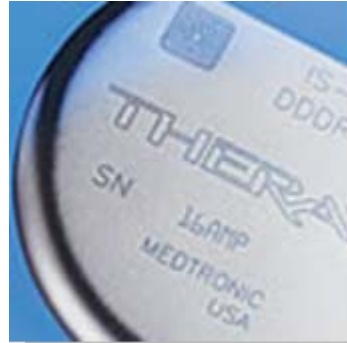
Text + data matrix marking on pacemakers
